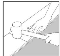
Start next row with the piece leftover (must be at least 300mm long), ensuring that end joints are staggered at least 300mm. Place the first plank of the new row with the tongue side matching the groove side of the plank in the previous row and then press it down with the help of a hand roller, or slightly tap with a rubber hammer.
