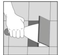
Try to remove the tile without damaging the subfloor. If this is not possible, the subfloor should be filled with a suitable levelling compound. Be caution with this, to ensure that the subfloor is completely flat and smooth.
