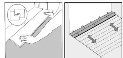
Cut the last plank to the correct width. Place the last plank on top of the second to last row and cut as indicated. Allow a 5mm to 10mm distance to the wall for the expansion gap. The width of the last row of planks should be equal or bigger than 5cm.
