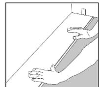
Hold the next plank tight to the short end of the first one matching the corner and then press it down with the help of a hand roller, or slightly tap with a rubber hammer. Make sure that the long sides of the planks make a straight line. Complete first row in the same way and cut final plank of the first row to the correct length. The distance to the wall should be 5mm to 10mm.
