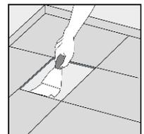
Use the recommended adhesive to glue the new tile into place. Follow the installation instructions. Press the tile down and place some weight on top of it while the adhesive dries. Avoid traffic immediately after to ensure perfect adhesion. Remove any surplus adhesive.
