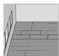
Make sure that the widths of the first and last rows planks are equal or bigger than 5cm (2") of the plank. If the wall is very uneven, cut the planks with the corresponding width to eliminate the unevenness. Place the first plank on top of the second row and cut as indicated. Or draw the outline of the wall by "sliding" a cut off-piece along the wall. Then cut the planks along the line.
