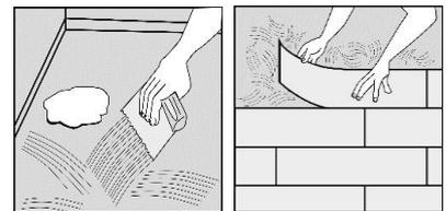
On wooden floors, we recommend laying Hydrocork crossways to the existing floorboard. Start installing in the right-hand corner with the tongue side of the plank facing the wall. The Hydrocork connection system is designed to be installed in a vertical connection by pressing from top to bottom (without making any angles). Maintain a gap between 5mm and 10mm from the wall.
